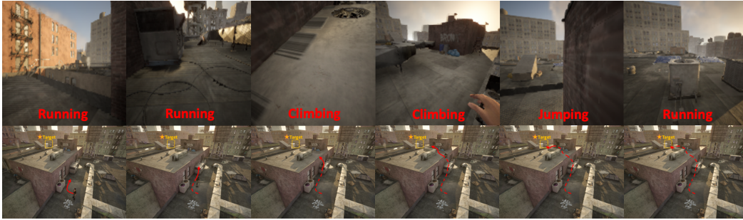
Figure 4: An exemplar sequence from the embodied navigation agent in the Roof . The RL-based agent learned to climb on a box and wall and jump over an obstacle to reach the goal location in a short path.
